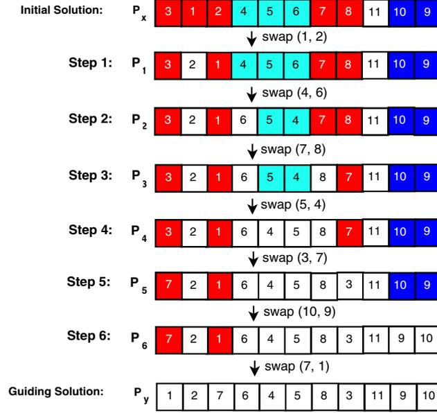
Fig. 4. Path generation for quadratic assignment problem
