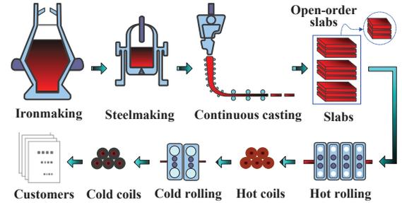
Fig. 1. Sketch of the production process of silicon steel.
